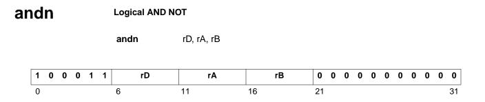
The contents of register rA are ANDed with the logical complement of the contents of register rB; the result is placed into register rD.
